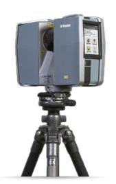
Time-of-flight range measurement: Pulsed
